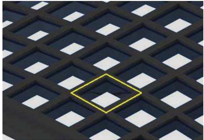
Figure 38. A damaged screen cell
